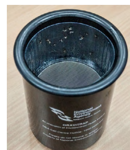
Figure 16: Gravitrapp with mosquitoes trapped on the sticky lining 24
